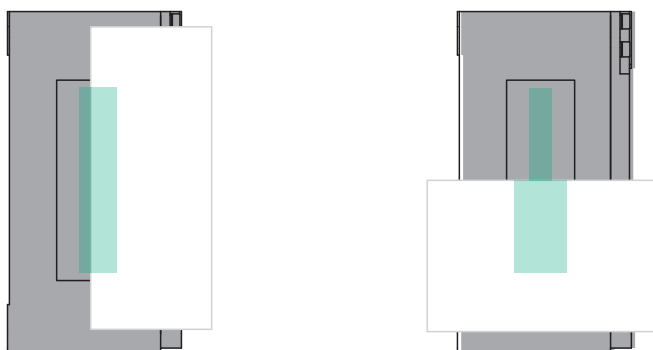
Fig. 4.12: Alignment check with projection screen (paper) in front of the receiver, vertical orientation on the left and horizontal orientation on the right
