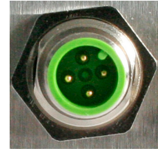
Fig. 25 Male connector on the IMC5420IP67-TH24 controller
